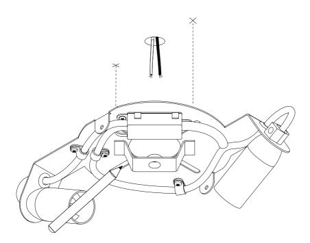
Drill holes and insert wall plugs. Ensure you use the correct type of drill and wall plug for the type of ceiling you are drilling into.
