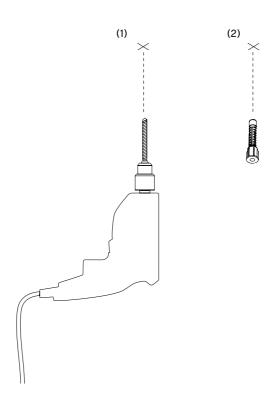
Screw the ceiling bracket into the ceiling, using the appropriate screws for the wall plugs used.
