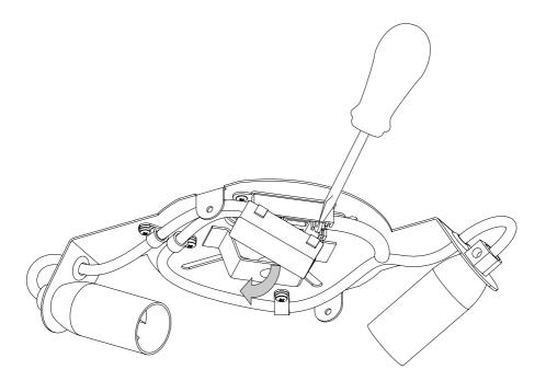
Loosen the two screws on the connector block, closest to the protective sleeve.
