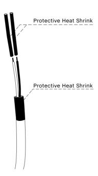
A heat gun can be used to shrink and fix the protective insulation in place, as shown below.
