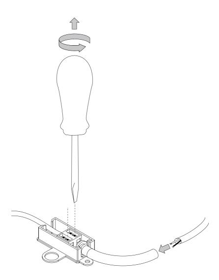
Feed the main cables into separate slots on the connector block. Insert the live mains cable into the side with the live cable on the lamp, and fasten the corresponding screw.
