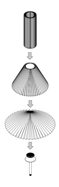
Once the shade is in place, gently adjust the pleats at the top so that they are evenly spread out, as shown below. Once the shade is as illustrated, the top screw can be fully tightened.
