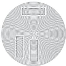
**PLANE SAWN:** The board has a lively appearance, the structure is in curves.
