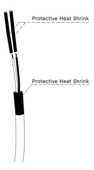
A heat gun can be used to shrink and fix this protective insulation in place, as shown below.
