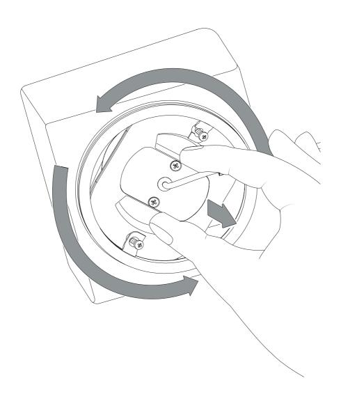
Place the light engine back into the glass shade and turn clockwise, locking the two screws into the hooks on the bracket.
