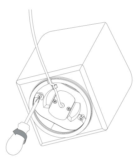
Turn the light engine counterclockwise until the two screws are free from the hooks on the bracket, tilt the light engine and pull it out from the glass shade. Now you can replace any broken parts with original HAY replacement parts.
