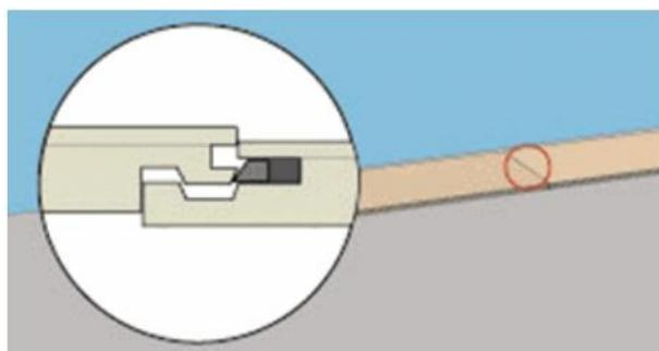
With Maxwear you install a floor with the most modern and easiest system to install on the market. The click system is called Rolloc 5G and is developed by Välinge Innovation <sup>1</sup> for Golvabia. The unique design of the short end of the board makes it possible to install the board in one simple movement without using any tools or chemicals.
