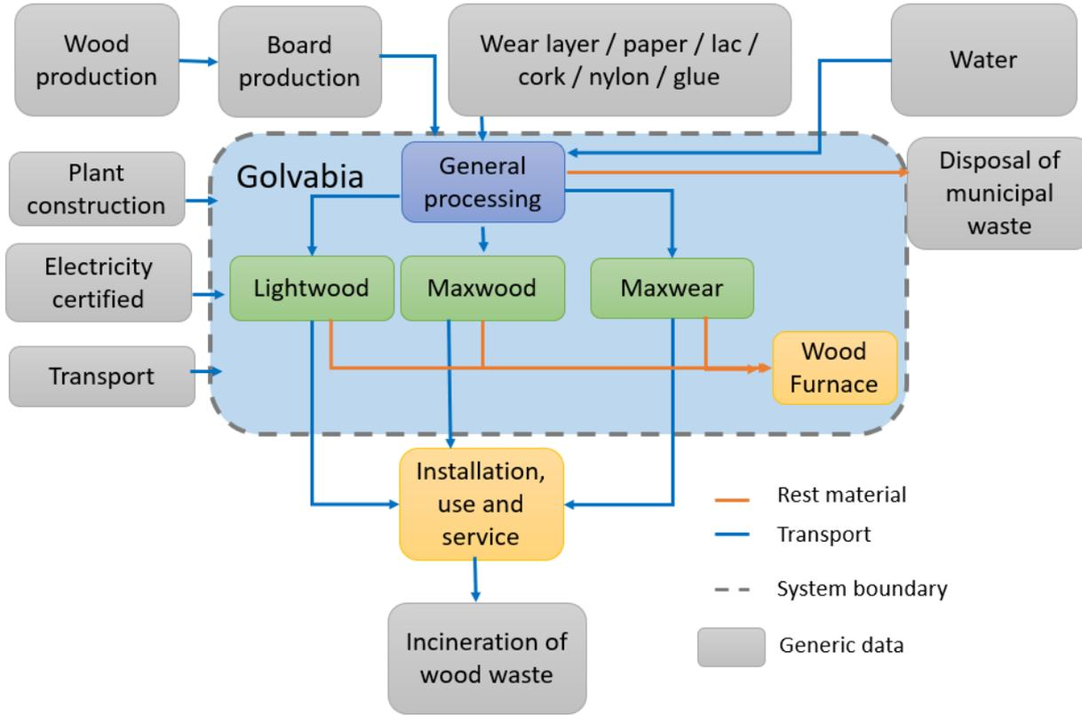
The image show system boundary (1), main processes and type of data quality used to represent these processes.
